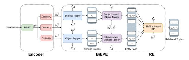
Figure 1: The Architecture of BiRTE. The modules with the same color have the similar inner structures. The solid lines represent the training process, and the dashed lines together with the solid lines represent the inference phase.
